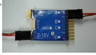
Whenever currents higher than **2** amps and up to **20** amps are required, *all* 4 plus pins need to get a separate power supply. Also the output (A,B,C and D) needs all 4 plus pins.
