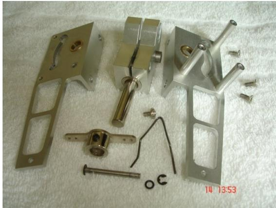
6. Nosewheel retract disassembled.
