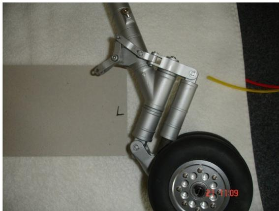
10. Left main gear pivot mechanism.
