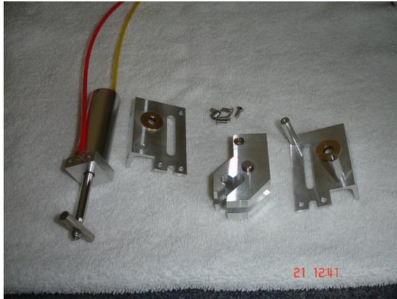
12. Main gear retract unit disassembled.
