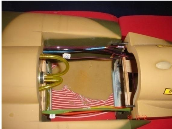
28. The nose section and main fuselage before joining.
