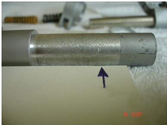
4. Point for another flat spot at the scissor link at bottom of nose gear.
