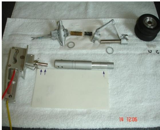
2. Nosewheel disassembled.
