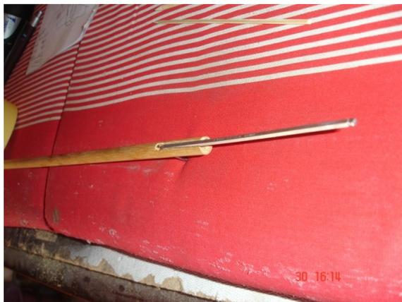
30. Dowel rod and hex key to ease the joining of nose section and fuselage. It was wrapped with isolation tape and was strong enough for the task.
