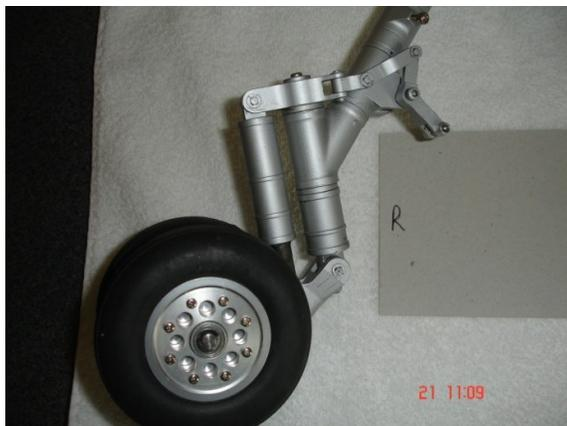
11. Right main gear pivot mechanism.
