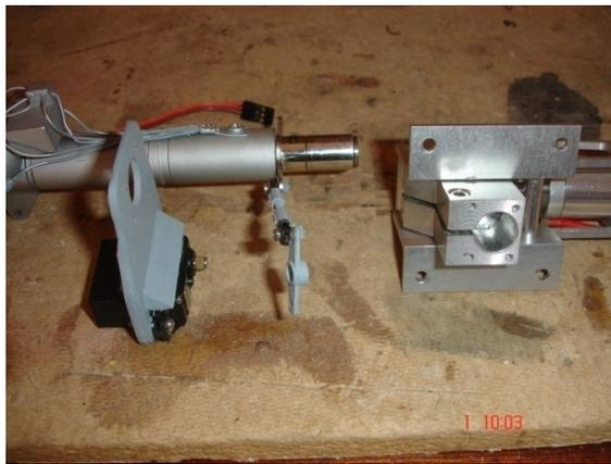
19. Bracket for direct nose wheel steering servo.
