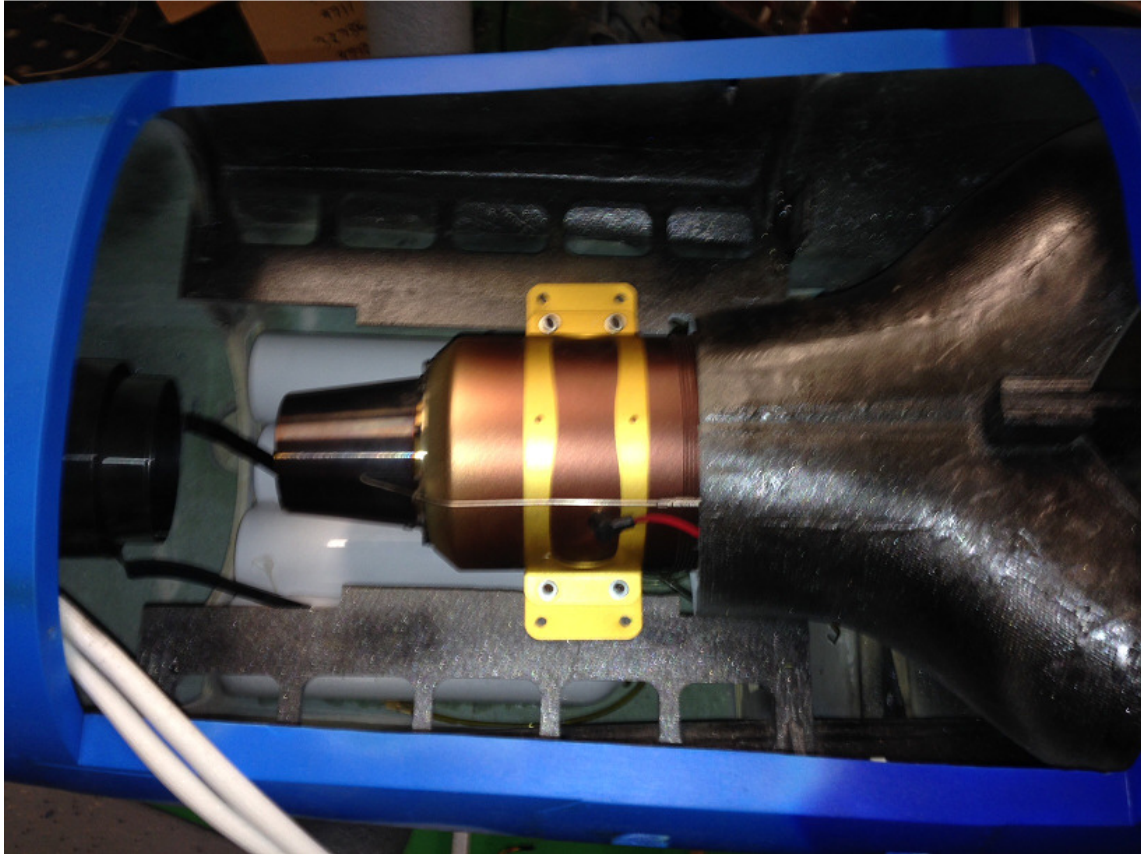
Photo 7&8 – mounting thrust tube, bypass and engine.
