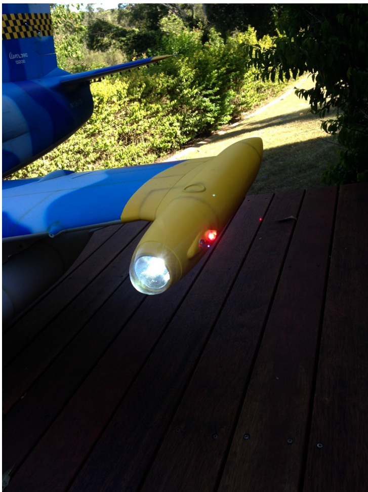
Photo 13: Landing lights installed from BrainCube (UK)
