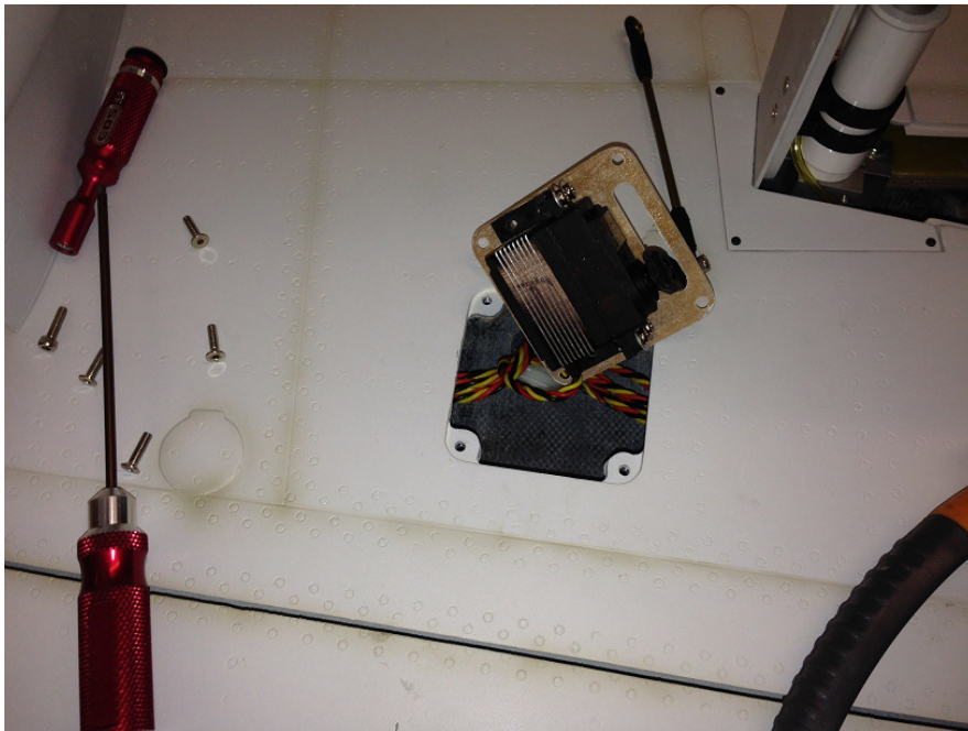
Photo 11&12 – Flap servo installation and pushrod.
