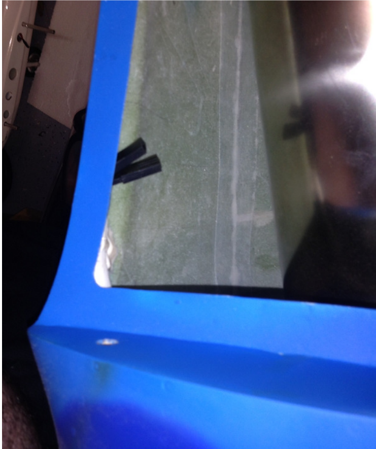
Photo 5 – Rear section with the tailplane and vertical stab removed and servo wires run to rear.
