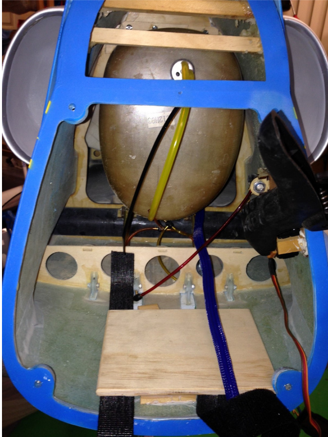
Photo 2 – Smoke Tank Layout added for Deisel. I used a normal Dubro tank for the smoke tank. (everything has not been secured yet so it looks messy)
