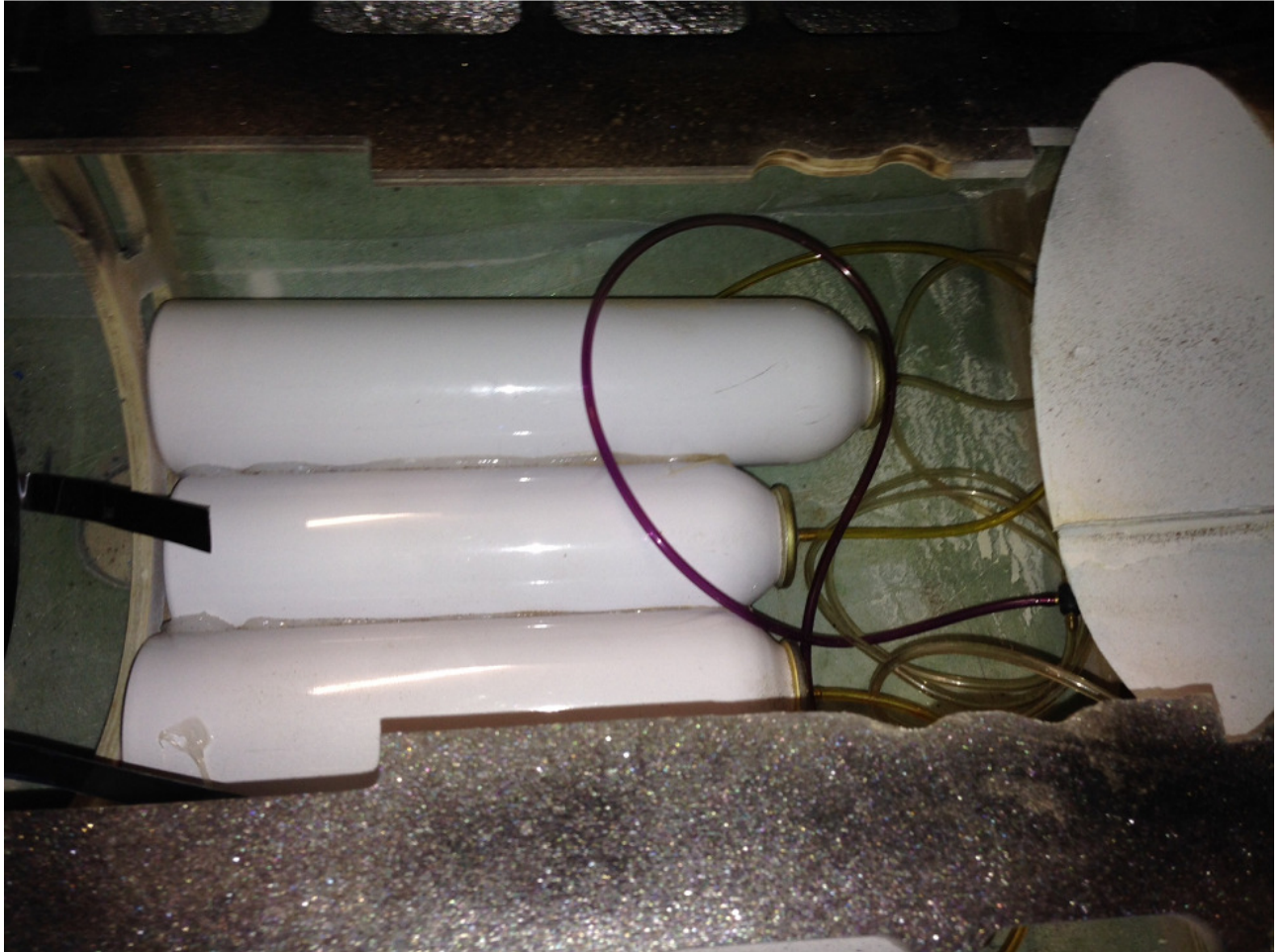
Photo 3 – air tanks installed under the engine bypass.
