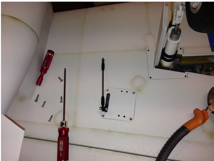
Photo 11&12 – Flap servo installation and pushrod.
