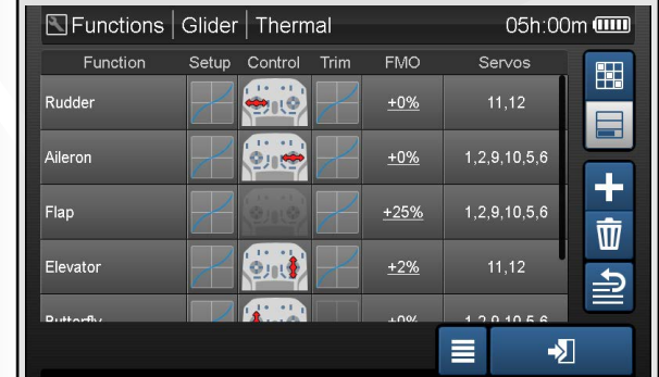
Flight mode Thermal: Flap and Elevator have a little offset
